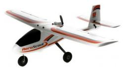
The plane is constructed of EPO foam and powered by a three-cell lithium-polymer battery. It has fully functional foam-molded control surfaces (ailerons, elevator, and rudder) as well as an electronic speed controller for the throttle. The rudder controls are linked to the plane's nose gear to permit control on the ground while taxiing. Assembly time, including binding the transmitter to the receiver, is about 30-minutes.
